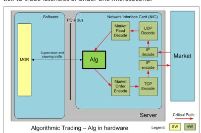
In the diagram to the left, the Alg has been redesigned as an FPGA HW solution and deployed within an FPGA on the NIC. The flow now goes direct from the Market Feed decoder through the Alg and on to the Market Order Encoder (if the Alg decides a trade is required).
